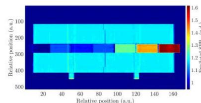
Cross-section of Gammex phantom with seven tissue-equivalent inserts showing predicted SPR
